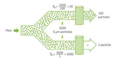
Generally a Beta Ratio at 5000 is accepted by the industry as being an 'absolute' rating for media prefilters.
