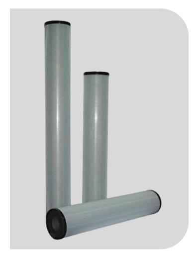
SS Series synthetic separator cartridges feature a specially developed hydrophobic synthetic media which offers all the permanent features of Teflon® screen, combined with ease of repair and lower cost. Synthetic mesh is wrapped around a treated, perforated metal shell, then adhesive bonded to gasketed metal end caps.
