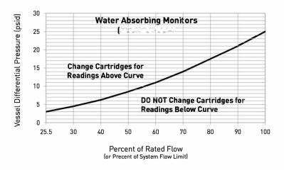
**EXAMPLE:** A 600 GPM vessel is operating at 300 GPM (50% of system flow limit). When the pressure differential reads less than 8 psid, the cartridges do not require changing. Should the pressure differential read 8 psid or higher, or if the cartridges have been in service for one year, the cartridges are due for changeout.
